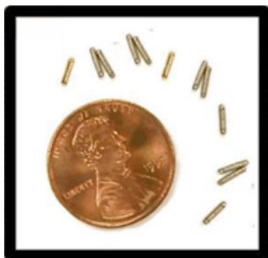
**Fig. 4.88.1: Brachytherapy seeds shown with a penny (19-mm diameter) for scale (modified from [579]).**
