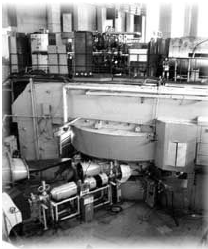
Fig. 4.116.1: Photo of the heavy ion cyclotron U-400 at JINR in which livermorium was synthesized. (Photo Source: Lawrence Livermore National Laboratory) [672].
